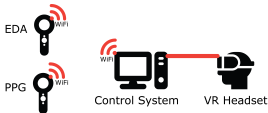
Fig. 2. The schematic overview of the SensCon. Data are acquired via PPG and EDA sensors in the VR controller. Physiological data are streamed within a UDP protocol to the experiment control PC. Finally, the VR environment is displayed to the user via a wired HTC VIVE headset.
