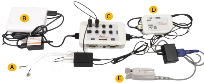
Fig. 5. The medical-grade system used as gold standards for evaluating SensCon-based EDA and PPG measurements. The EDA electrodes (A) and PPG finger clip sensor (E) are connected to the AUX ports of the Sensor & Trigger extension (STE) (C). For signal amplification and streaming to the acquisition PC, we use a LiveAmp amplifier (D) and a power bank for energy supply to the STE (B). All components were placed inside a pouch and comfortably worn by participants across the experimental sessions
